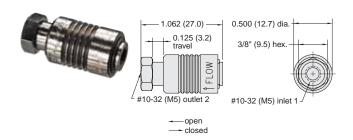
Medium: AirMounting: Inline or direct to fittingStem Travel: 1/8" (3.2)Material: Nickel plated brass
